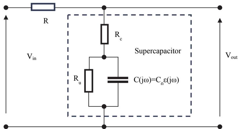
Figure 8. Scheme of the voltage divider
