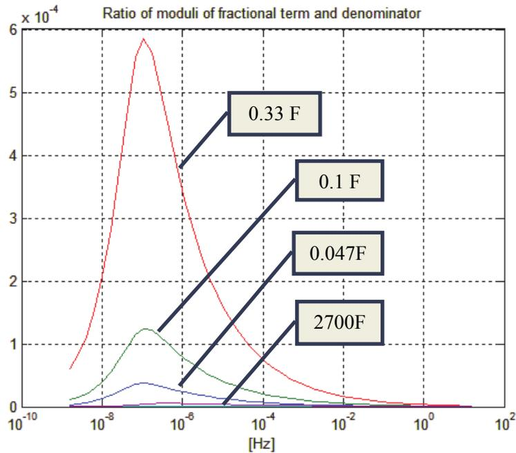
**Figure 4.** Frequency dependence of ratio  $S$  (18) for various supercapacitors
