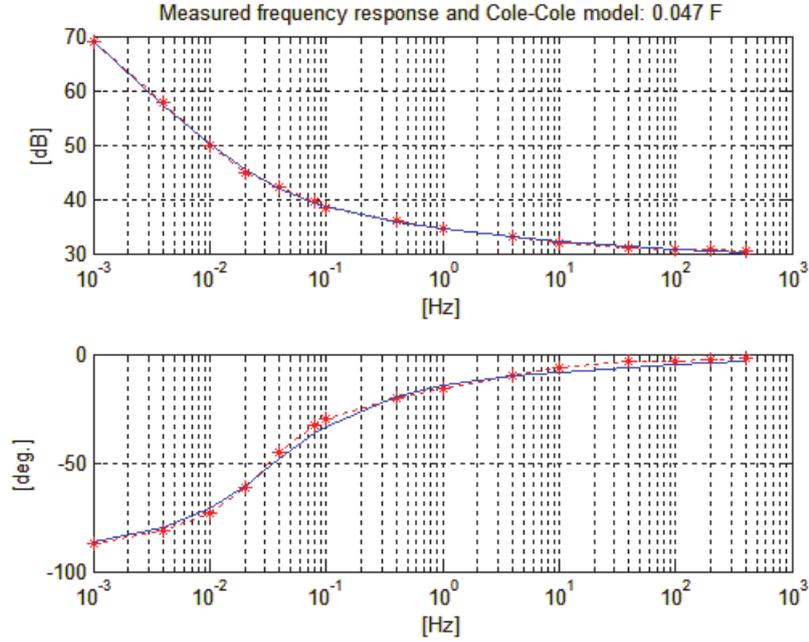
**Figure 3.** Measured frequency response points (asterisks) and approximating function (17) for 47 mF supercapacitor
