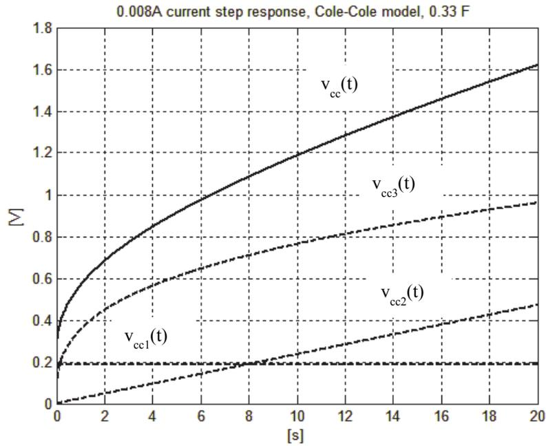
Figure 7. Current step response of supercapacitor of 0.33 F
