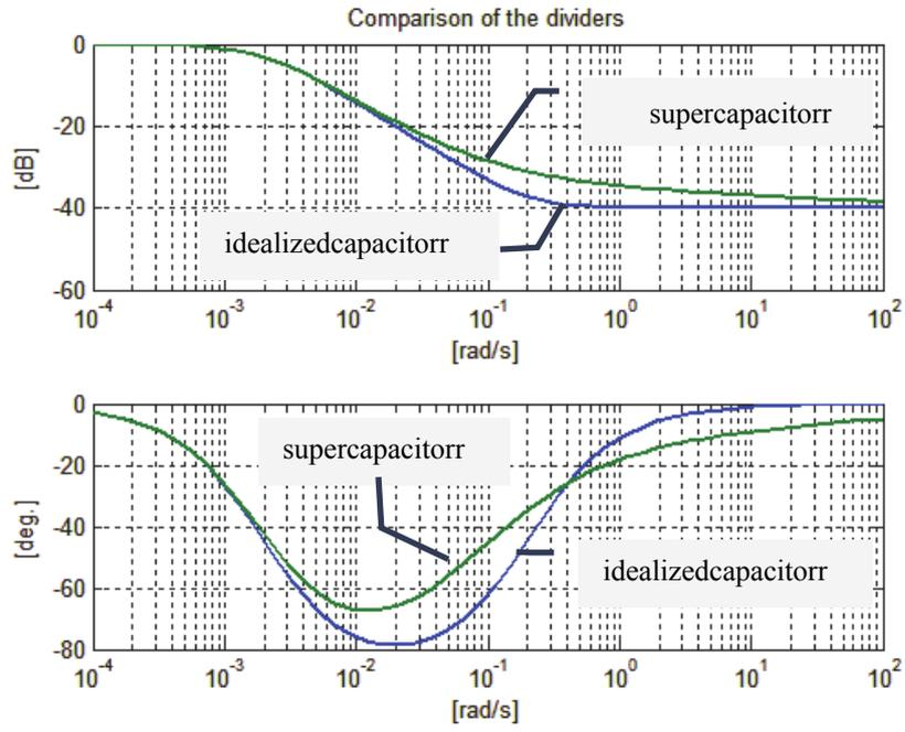
**Figure 9.** Bode plots of transfer functions of the dividers with supercapacitor and idealized capacitor
