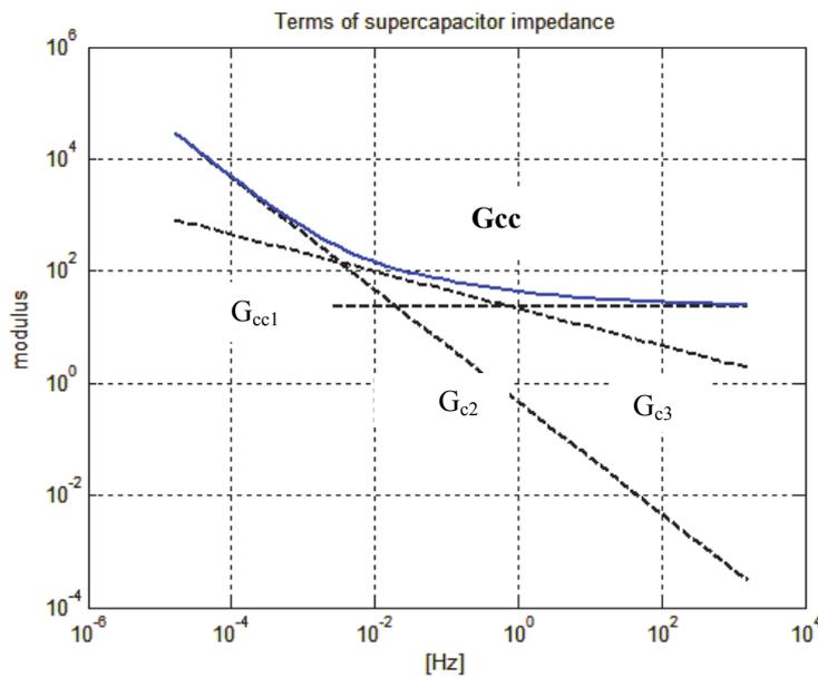
**Figure6.** Moduli of terms of equation (22) and modulus  $G_{cc}$  for supercapacitor 0.33 F
