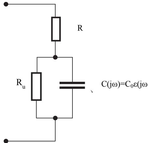
**Figure1.** Equivalent circuit of supercapacitor
