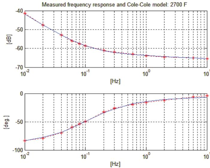
**Figure 2.** Measured frequency response points (asterisks) and approximating function (16) for 2700 F supercapacitor
