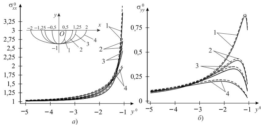
**Figure 6.** Stresses  $\sigma_{xx}^0$  and  $\sigma_{yy}^0$  on the extension of the symmetry axis of the notch along the arc of the ellipse for  $\delta = 1$  and various values of  $l$
