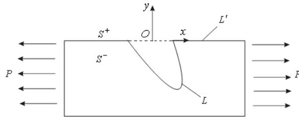
**Figure 1.** Plate element with notch under uniaxial loading
