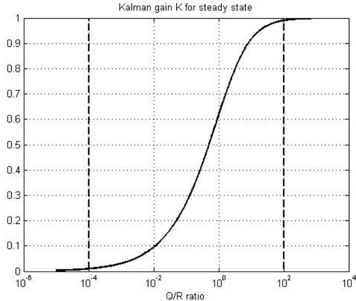
**Figure 1.** Kalman filter gain vs.  $Q/R$  ratio
