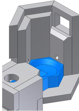
**Figure 4.** Internal construction of plasma reactor – CAM model
