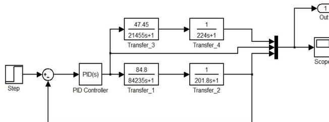
**Figure 6.** Mathematical model of plasmotron reactor system
