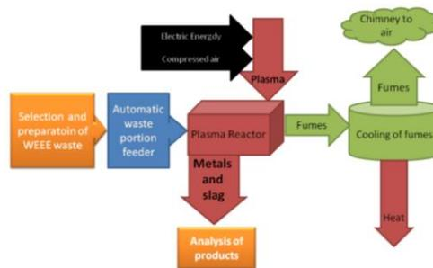
**Figure 2.** Block diagram of the designed process for research over high temperature plasma technology for metals recovery and electronic waste utilization
