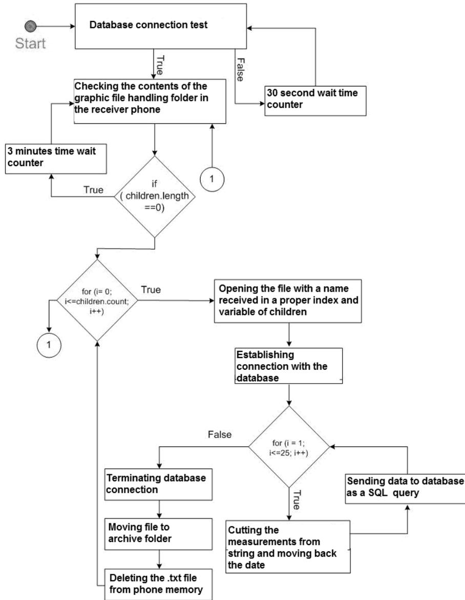
**Figure 8.** Simplified algorithm of the Receiving Station – computer – application
