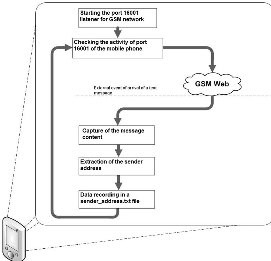
Figure 5. Receiving Station – mobile phone – operating diagram
