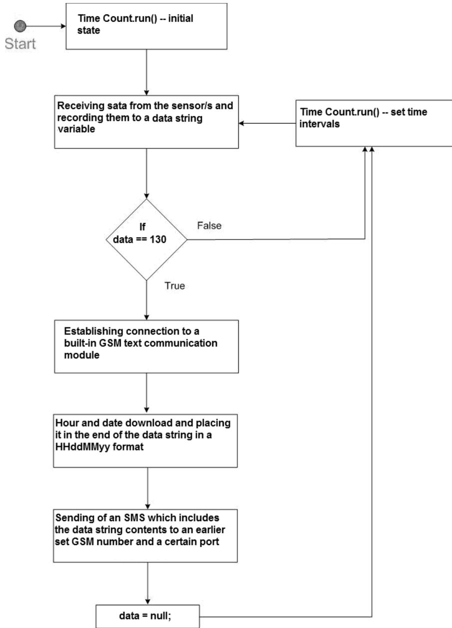
Figure 4. Simplified algorithm of the Broadcasting Station functioning
