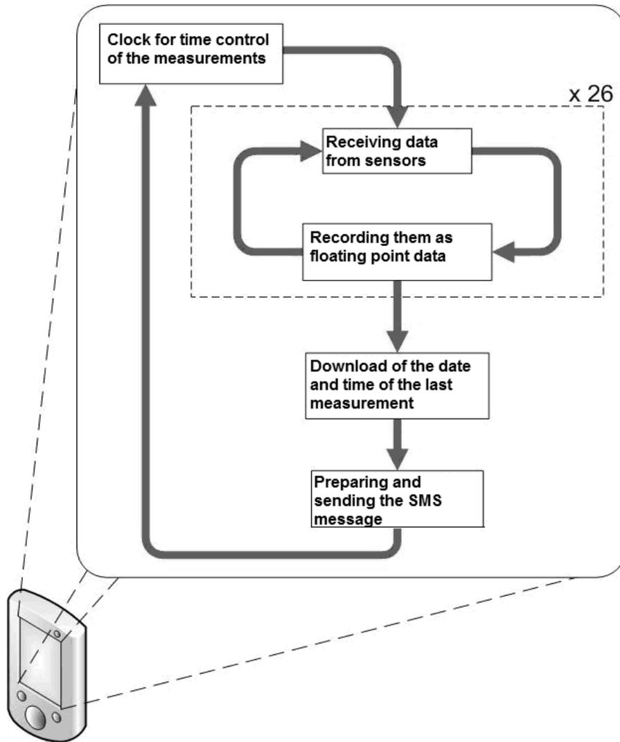
**Figure 3.** Broadcasting Station program operation diagram
