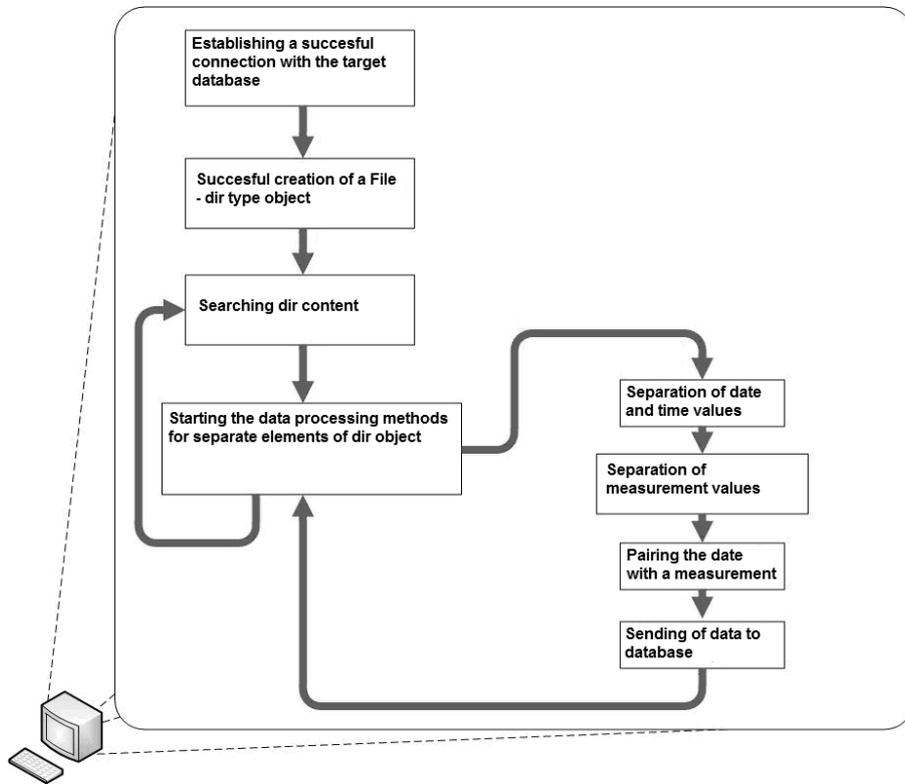
Figure 7. Receiving Station – computer – operating diagram
