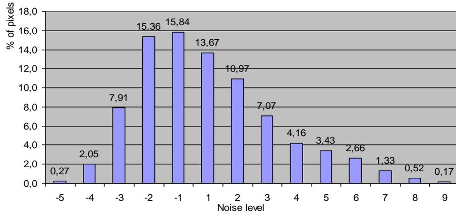
**Figure 8.** Noise distribution in images acquired using combination of NG4 5,0 mm and BG38 1,0mm filters (filter 2).
