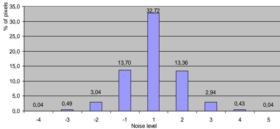
**Figure 6.** Noise distribution in images acquired without filter usage (filter 0).
