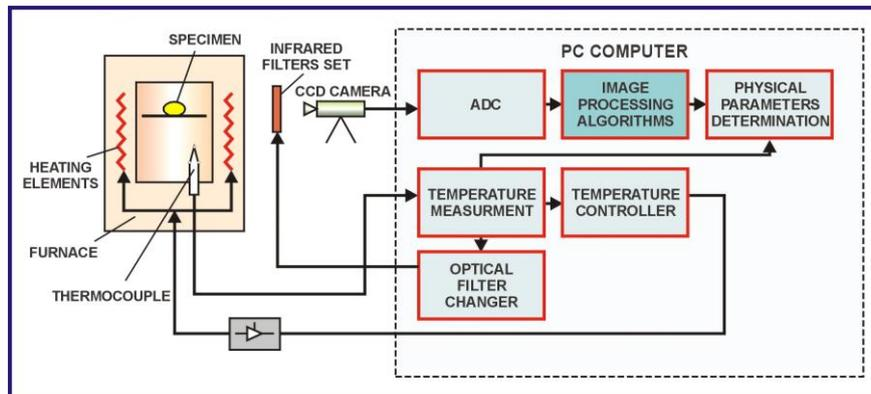
**Figure 2.** Block diagram of the "THERMO-WET" measurement system.
