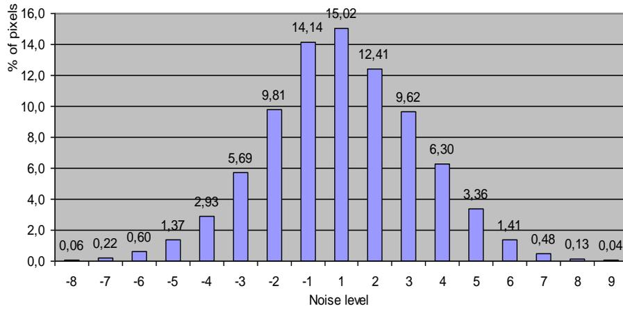
Figure 7. Noise distribution in images acquired using NG4 2,5 mm filter (filter 1).
