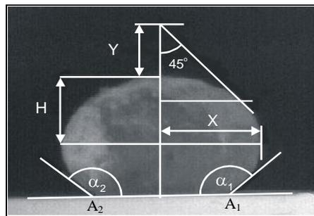
**Figure 4.** The exemplary specimen with important geometric parameters marked.
