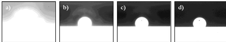
**Figure 5.** Aura phenomena – infrared filters selection influence. High temperature images of palladium 1564°C (a-no filters, b,c- incorrect infra-red filters selection, d-proper filters selection).
