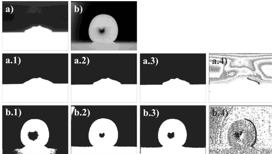
**Figure 2.** Results of image thresholding; a) image of palladium, 15500C; b) image of glass, 8900C; 1) global thresholding,  $T = 170$ ; 2) global thresholding with iterative threshold selection; 3) local thresholding with iterative threshold selection; 4) local thresholding with threshold set to median.
