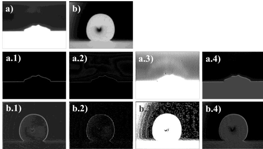
**Figure 3.** Results of edge-based image segmentation; a) image of palladium, 1550<sup>0</sup>C; b) image of glass, 890<sup>0</sup>C; 1) Sobel's masks; 2) Laplace's operator; 3) Frei-Chen's masks; 4) Krish's masks.
