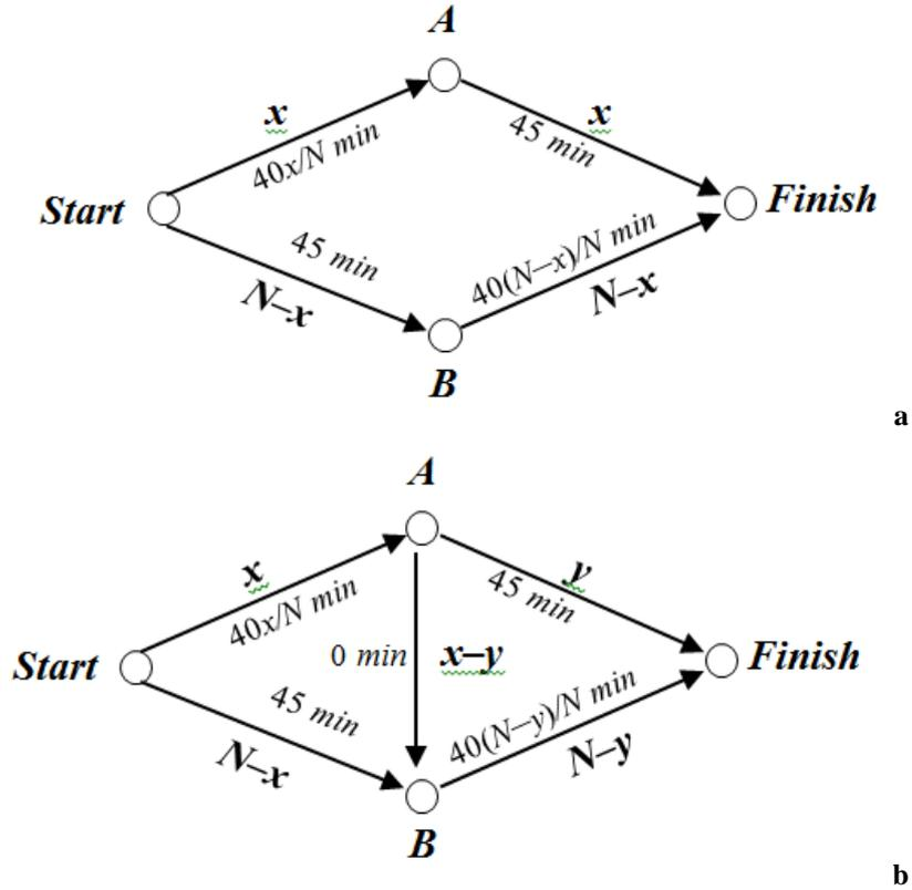
**Figure 1.** Time and number of vehicles on the route network with (A) and without (B) the additional connection *AB*
